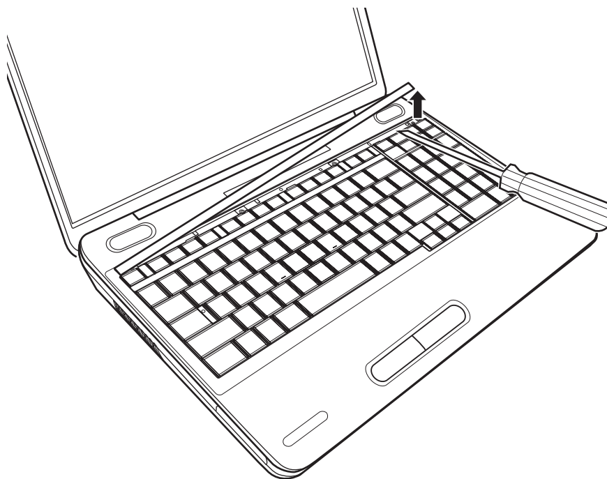
Figure 4.8 Removing the keyboard cover
